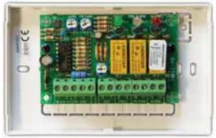
The SMART420MA module interfaces any 4-20mA output gas detector with any control panel.
