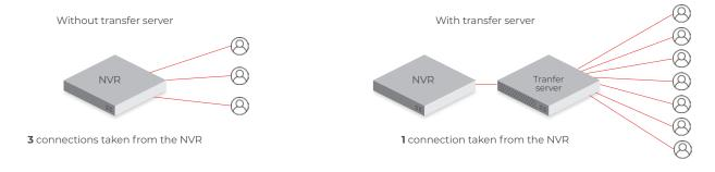
3) The Transfer Server will mirror all the devices assigned to it, so the "Quick Add" Device List will be fully populated as if the management server is in the same LAN as the IPCs.
